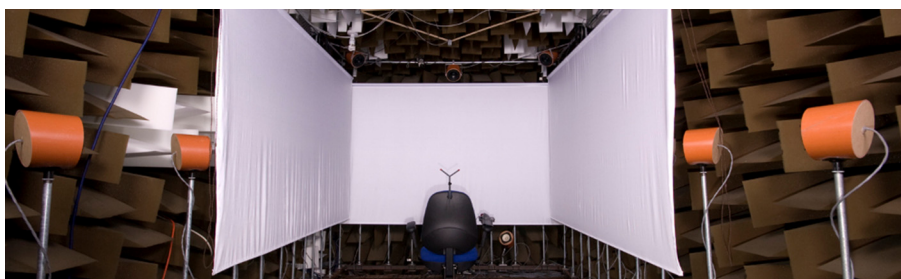
Figure 3 Testing apparatus. The apparatus that will be used to assess the sound localisation accuracy and speech understanding of patients in the trial. An array of loudspeakers and a visual projection system are positioned within an anechoic chamber. Thirty-six loudspeakers are distributed horizontally around the listening position with an additional 6 loudspeakers suspended above the listener and a further 6 loudspeakers positioned below the listener. The three visual projection screens are driven by three high-definition projectors. Responses are recorded using a trackball (localisation task) or through an intercom (speech understanding task).
